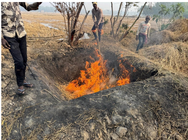
Figure 2: Example of well-constructed soil pit kiln with raised edges for safety
